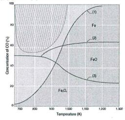
Figure Q1c. The Fe-O-C diagram. One line is missing.
