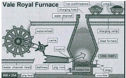
Figure Q1a. Layout of a typical 18th century blast furnace in England.
